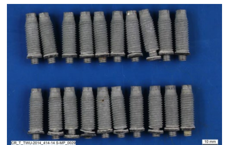
Removed S-BT fasteners after 12 weeks EN ISO 16701 cyclic corrosion test. No visible corrosion.
