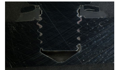
Polished cut image: activated Micro encapsulation on the tapping thread of the S-BT fastener
