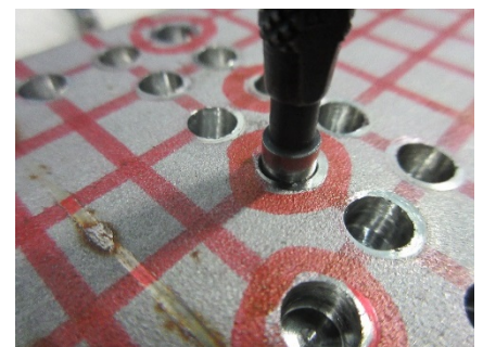
Testing of pilot hole quality
