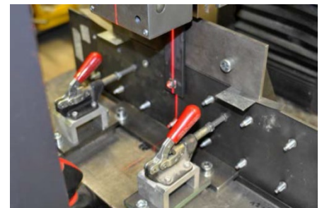
Test set up for shear load testing
