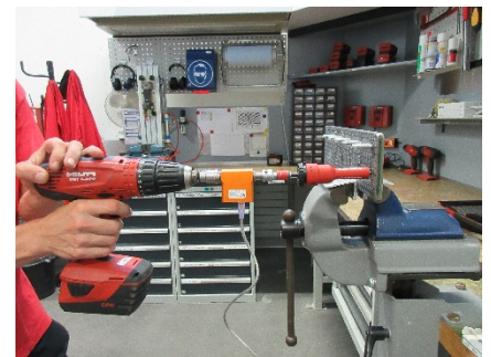
Test setup to test the forming torque of the studs in stainless steel base material
