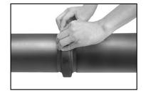
5. BRING THE MATING PIPETOGETHER: Bring together and align the two pipe ends to be joined. Slide the gasket over the ends and center it between the grooves of the pipe to be joined. No part of the gasket should protrude into the groove of either pipe.
