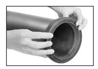
4. INSTALL GASKET: Install the gasket over one end of the pipe so that the pipe end is exposed. No part of the gasket should overhang this end of the pipe.
