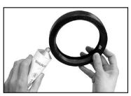
3. LUBRICATE GASKET: To help insert pipe smoothly and mount couplings smoothly without pinching, apply a thin layer of Shurjoint Lubricant to the sealing lips of the gasket and as well as to the exterior of the gasket. Other compatible lubricants may be used so long as they are not harmful to the gasket. System temperature should also be considered when selecting a lubricant. See page 40 for details.
